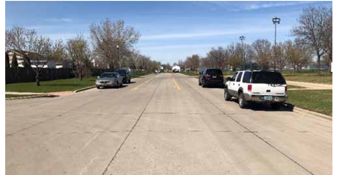
▲ Parents park in 18th Street S travel lanes during arrival and dismissal, forcing through traffic to drive in the center turn lane and creating visibility issues at the crosswalk.
