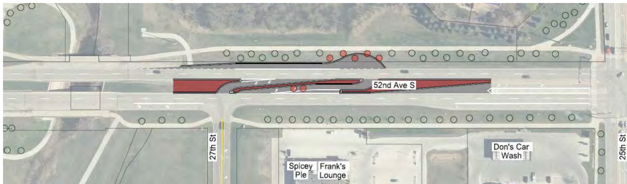
Figure 42 – 27th St & 52nd Ave Intersection - RCUT Alternative
