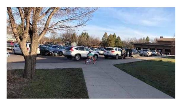
▲ There is no vertical separation between vehicle and pedestrian space, which results in drivers encroaching onto the sidewalk.
