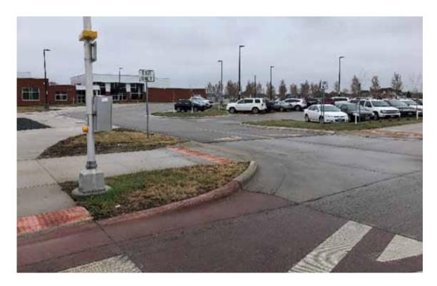
▲ Drivers do not stop or slow down when exiting driveway/turning across crosswalk. There is no signage or pavement markings.
