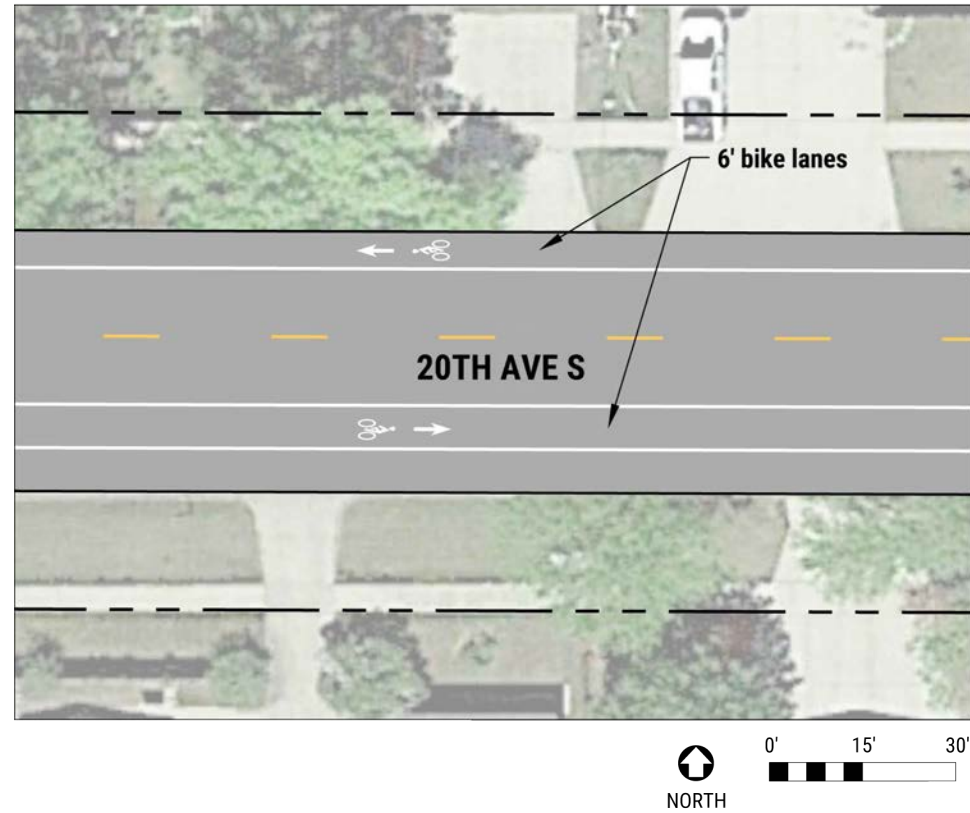
Alternative Concept Typical Section // 20th Ave S, Looking West
