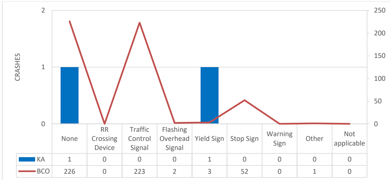
Figure 30 Heavy Vehicle Crash Severity by Intersection Traffic Control Device (intersection crashes only)
