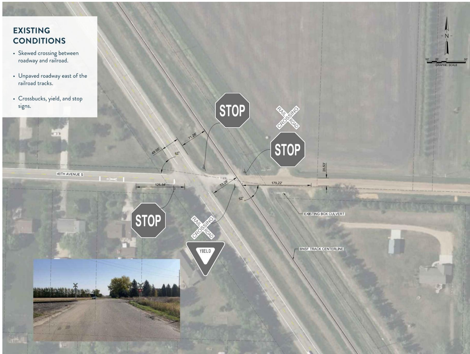
Figure 17-2: 40th Avenue S Existing Condition
