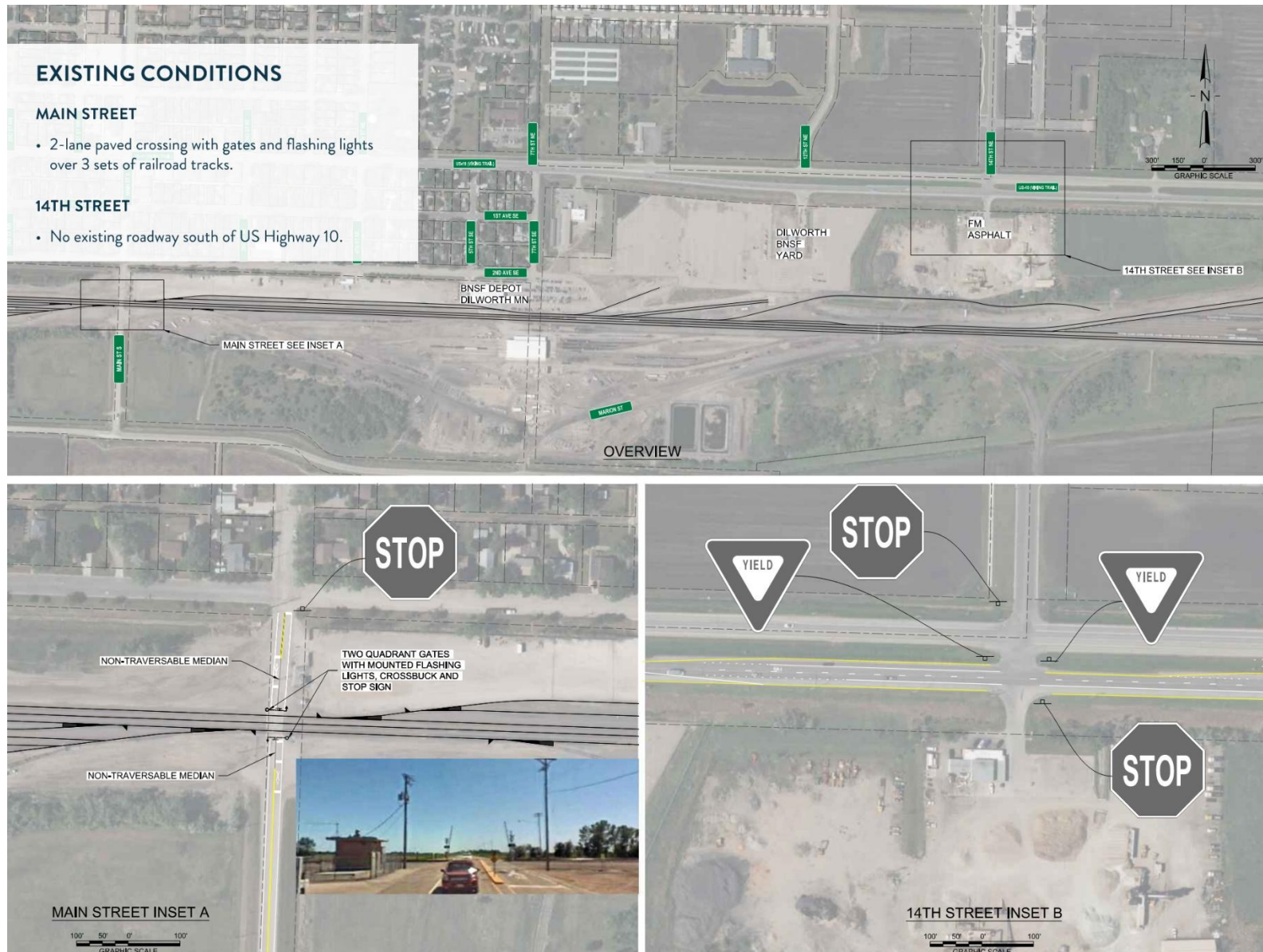
Figure 16-2: Main Street & 14th Street Grade Separation Existing Conditions
