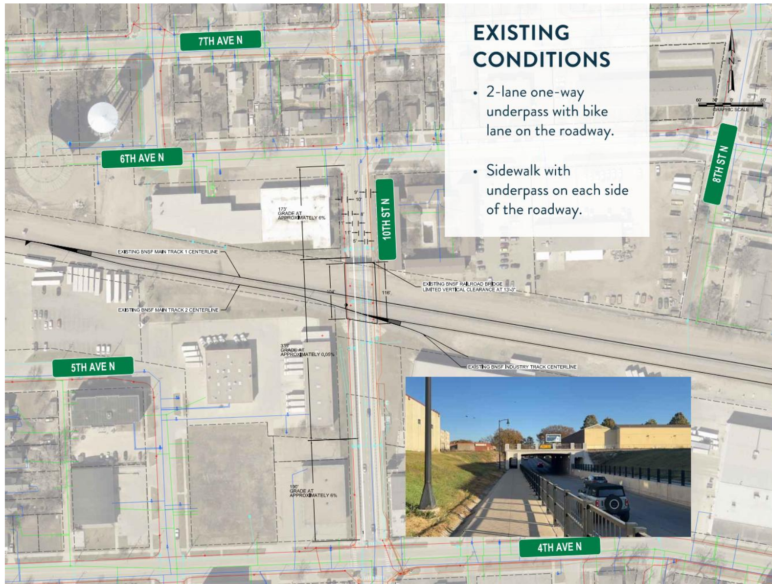
Figure 13-2: 10th Street Near 7th Avenue N Existing Conditions
