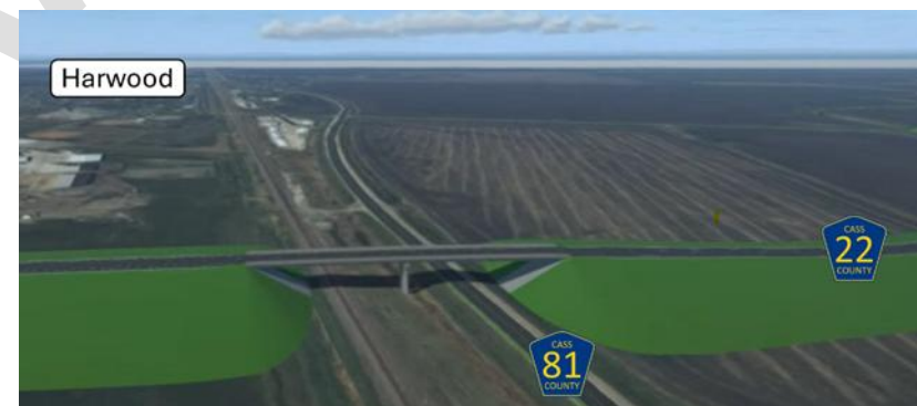
Figure 20-3: Realigned County Road 22 Overpass Concept
