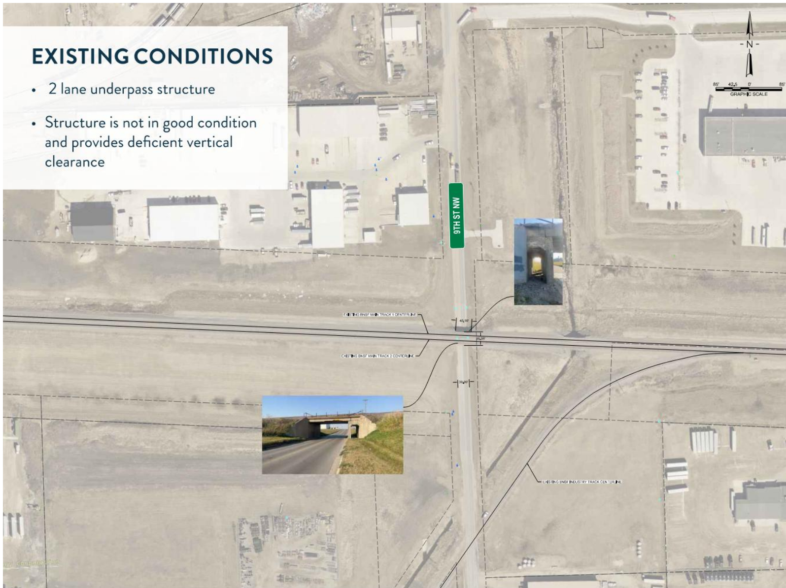
Figure 8-2: 9th Street NW Existing Conditions
