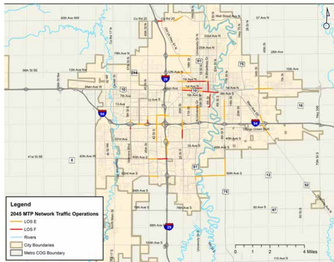
FIGURE 12.13: FUTURE 2045 FORECAST PLANNED NETWORK TRAFFIC OPERATIONS
